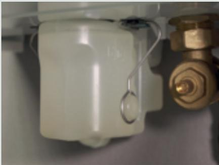
Figure 1: Original retaining clip and lugs
